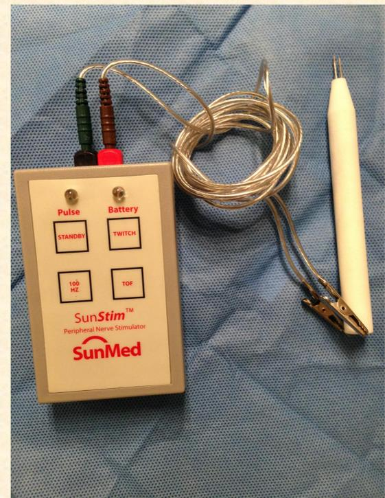
**Figure 3. “Beta” prototype probe and wiring compatible with autoclave sterilization.**
