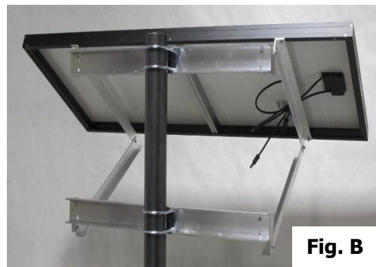
Note in Fig. B, the bottom channel has been moved farther up the post than in Fig. A to achieve a more horizontal adjustment for the panel.
